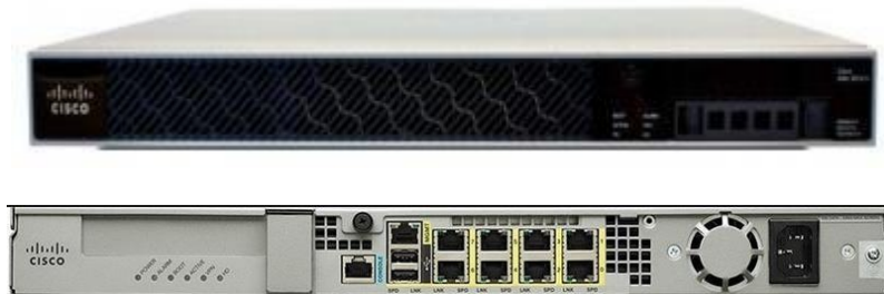
Figura 15 Cisco ASA 5525 Series Firewall (Front and Back).
