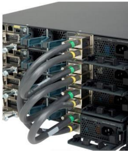
Figura 14 Cisco Catalyst 3560 – StackPower Connector
